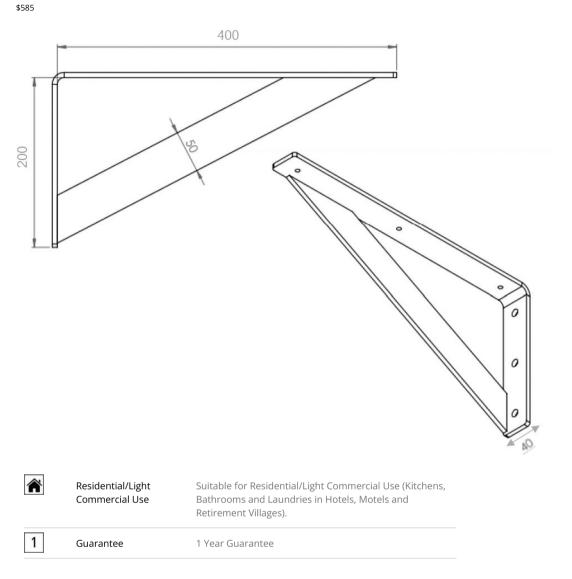
Wall brackets allow the basin/flat top to be wall hung without cabinetry. It is recommended that the bracket be fixed to the basin with an adhesive sealant. Bracket must be fixed securely to a stud on either side of basin.
